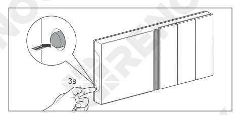
Press and hold the Power Button on Renogy ONE for 3 seconds to power it on or off.
