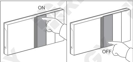
2. Press the panel switches to power on/off external loads.
