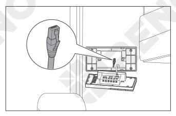
2. Reserve the RJ45 connector of the communication cable into the installation hole.
