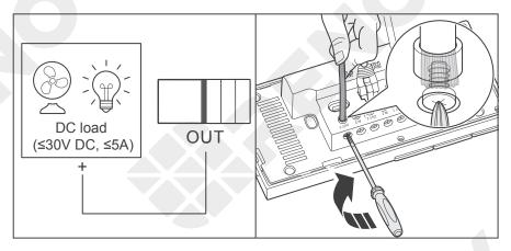
5. Insert the reserved tray cable connecting to the positive terminal of the load (appliance) into the Renogy ONE output terminal (OUT), and use a Phillips screwdriver to turn the wire hatch screw clockwise.
