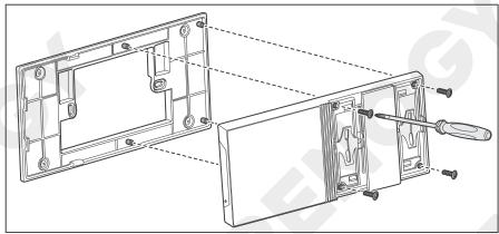
Put Renogy ONE on the base, and drive in the four M2 screws with the Phillips screwdriver #1 through the mounting holes to fix the Renogy ONE on its base.
