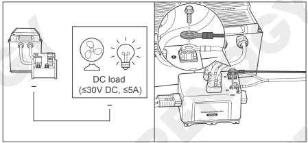
Connect one of the ring terminals of the tray cable to the negative terminal of the DC power supply, and connect the other end to the negative pole of the load.
