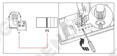
7. Insert the reserved end of the tray cable into the Renogy ONE input terminal (IN), and use a screwdriver to turn the wire hatch screw clockwise.
