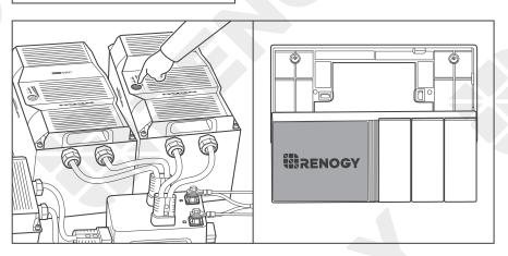
3. Power on the DC power supply and check if Renogy ONE automatically turns on with the LCD lighting up.
