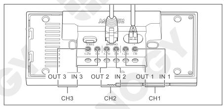
Ensure that the DC power supply cable and the cable that is connected to the positive pole of the load (appliance) are connected to the same group of terminals. For example, "IN 1" and "OUT 1" are in a group.
