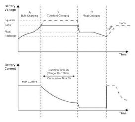
**Bulk Charge:** This algorithm is used for day to day charging. It uses 100% of available solar power to recharge the battery and is equivalent to constant current. In this stage the battery voltage has not yet reached constant voltage (Equalize or Boost), the controller operates in constant current mode, delivering its maximum current to the batteries (MPPT Charging).
