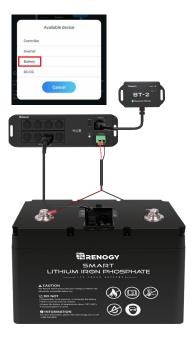
Before connecting the next device, disconnect the previous device from the SECONDARY port; Repeat Step 3 to connect another
