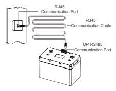
If you are using the monitoring screen with a parallel battery bank, the battery management systems of paralleled batteris must be connected to enable proper communication with the battery bank. Please connect the LINK RS485 Communication Ports of the former batteries to the UP RS485 Communication Ports of the latter ones using CAT5 (or above) Ethernet cables (not included).
